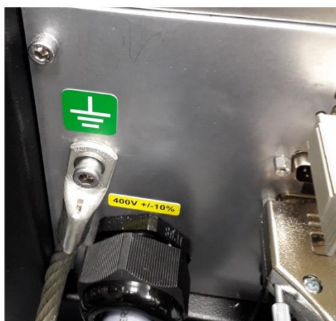
Connection of braided lead 091-1067-00 to ground stud at rear of DC PSU. Connect opposite end of braided lead to the end-user's installation frame ground
